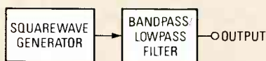
FIG. 7—LOWPASS OR BANDPASS FILTERS can clean up a squarewave source and provide a pure sine wave output.
